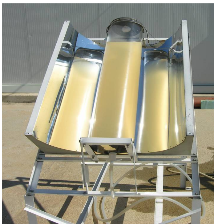
Figure 5.1 Enhanced SODIS batch reactor (EBR) filled with E. coli K-12 contaminated turbid water.
